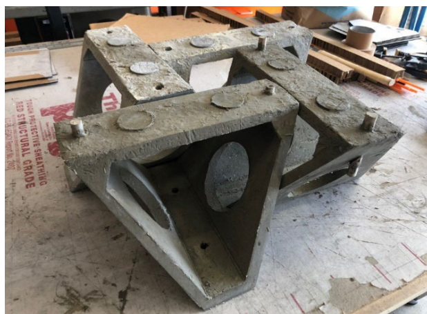
Prototype of mudflat reef element for the Reef Design Innovations for Living Shorelines project.
